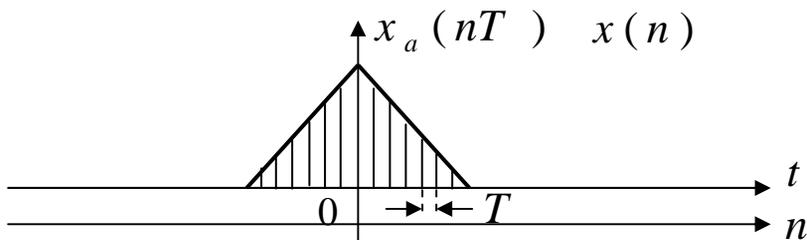
$$x(n) = \frac{1}{2\pi} \int_{-\pi}^{\pi} X(e^{j\omega}) e^{j\omega n} d\omega$$
